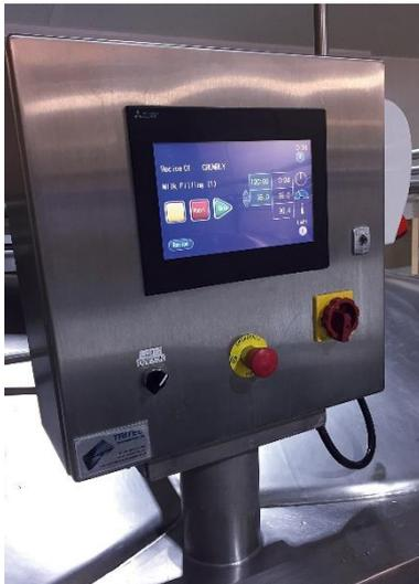
**Image 2:** With the new Mitsubishi Electric GOT2000 Human-Machine Interface (HMI) Dewlay's cheesemakers can now monitor the different cheese vats simultaneously, receive alarms as well as adjust the processes parameters in real-time and according to their expertise.
