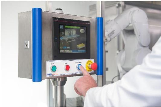
**Image 3:** A GOT2000 HMI enables operators to easily set what type of cutting is required and monitor the process.
