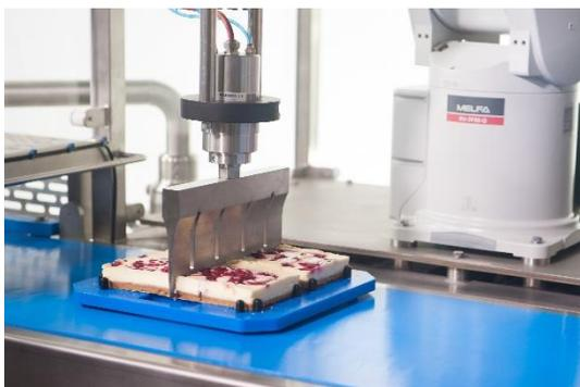
**Image 4:** The robots can perform quality slicing by means of state-of-the-art ultrasonic blades from Telsonic.
