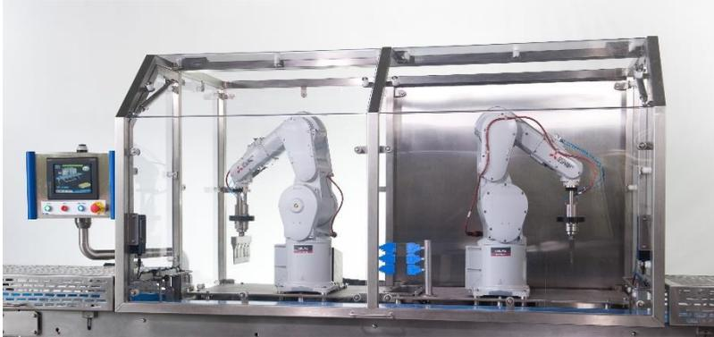
**Image 1:** A big contributing factor in the machine's versatility are two robotic arms from Mitsubishi Electric, which can attune to the line speed and do all the necessary cuts on the move.
