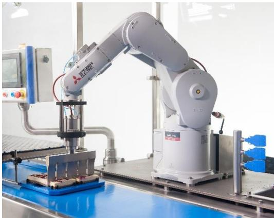
**Image 2:** Mitsubishi Electric's RV-F series of six-axis robots offers class-leading speed, precision as well as IP65 ingress protection for food grade wash-down working environments.
